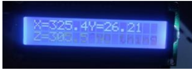
Figure (14) Accelerometer values on LCD screen
