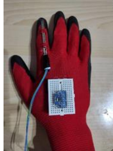
Figure (11) the installation of a flex sensor and accelerometer on the glove
