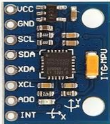
Fig. (4) MPU6050 accelerometer.
